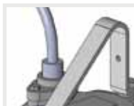
Power cable insulation treatment. No water leaking.
