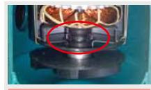
Oil to cool down the Mech seal
